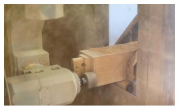
State of the Art CNC Machines in Our Ellington, CT Manufacturing & Design Facility CNC Machine Shaping a Tenon
